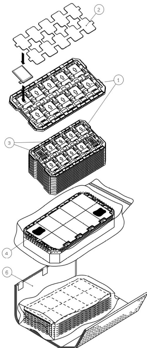
Step 1. Each product is to be placed in one of the cut-outs of the tray with the display surface facing upward.
