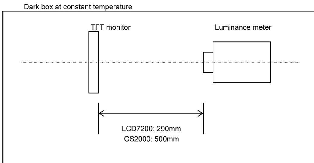
Measurement is made after 30 minutes of lighting of the backlight.
