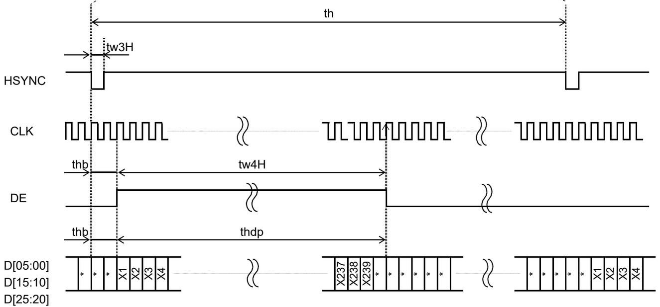
9.3 Input timing example (fCLK = 5.0MHz、5.6MHz、6.25MHz)
