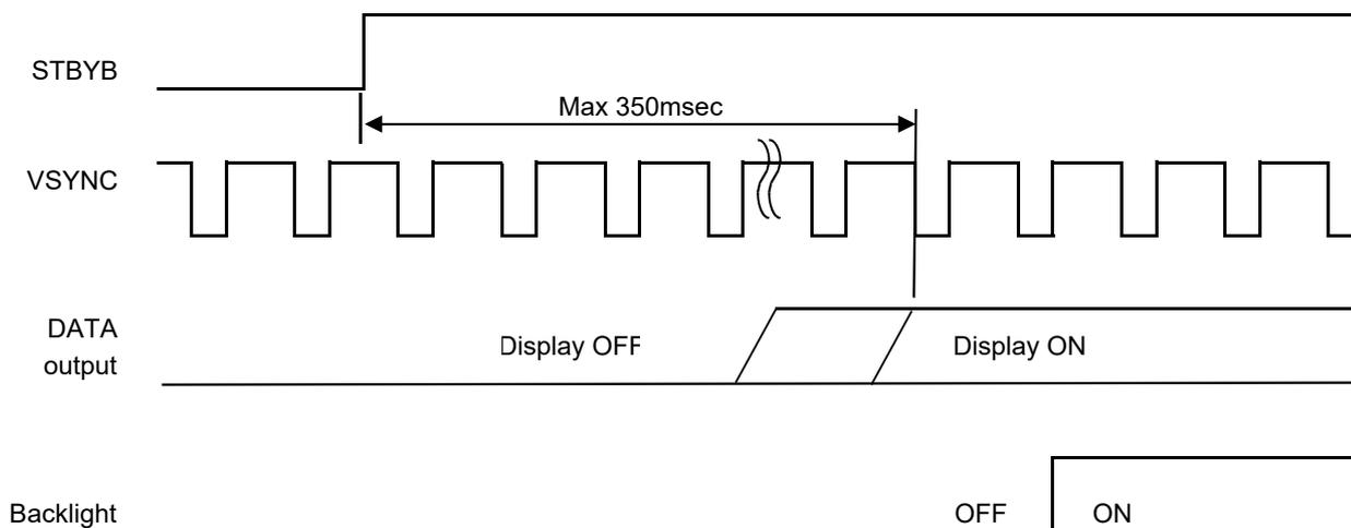
The following time will be needed by the time the standby sequence is ended from the standby setting.
