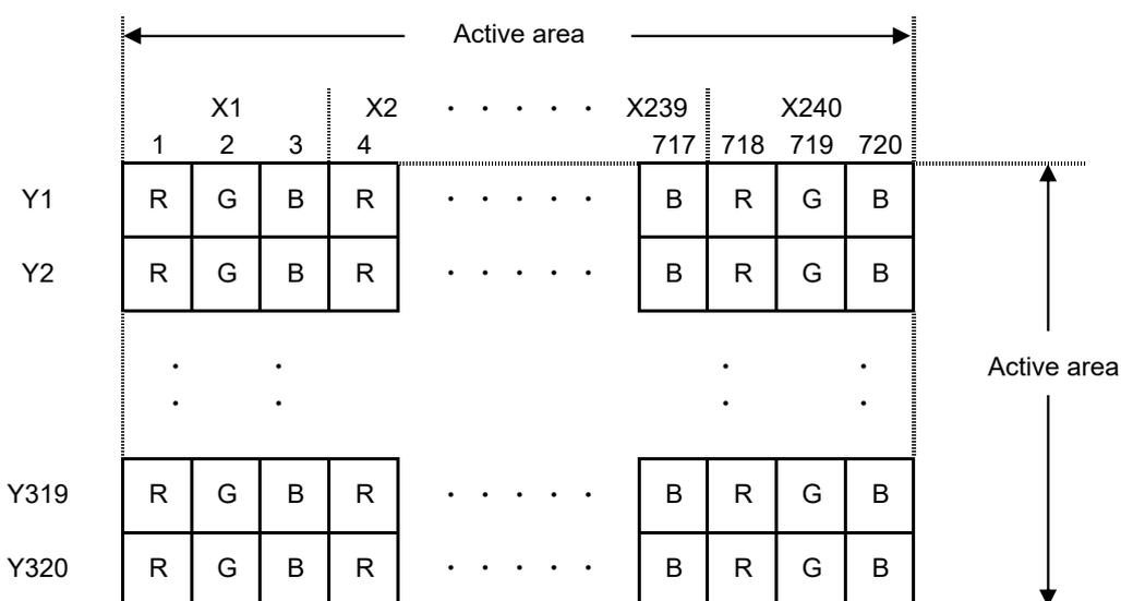
Dot arrangement (FPC cable placed left side)
