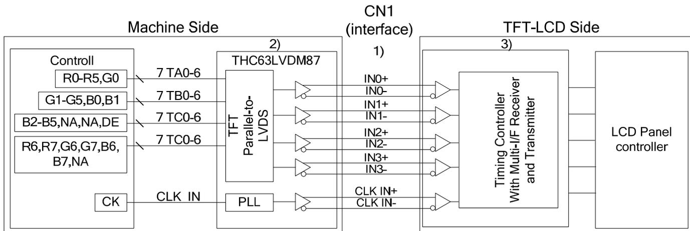
Note 1: LVDS cable impedance should be 100 ohms per signal line when each 2-lines (+, -) is used in differential mode.
