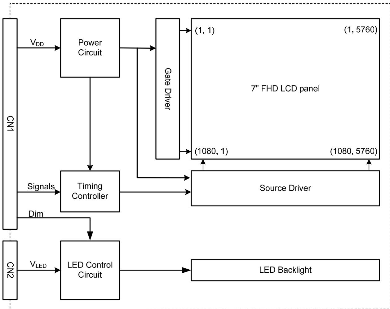
Note 1: Signals are CLK and pixel data pairs.
