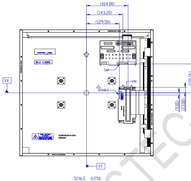
LED DB connector: CI0114M1HRL-NH(CviLux) or equivalent
