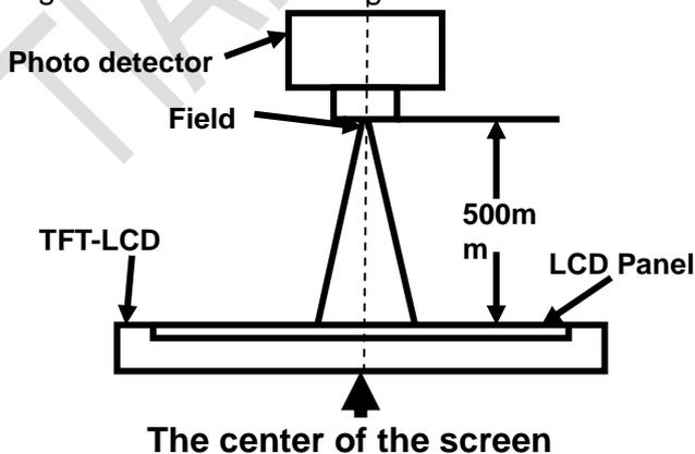
Note 2: Definition of viewing angle range and measurement system.
