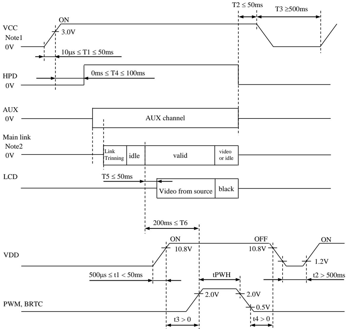
Note1: If there is a voltage variation (voltage drop) at the rising edge of VCC below 3.0V, there is a possibility that a product does not work due to a protection circuit.
