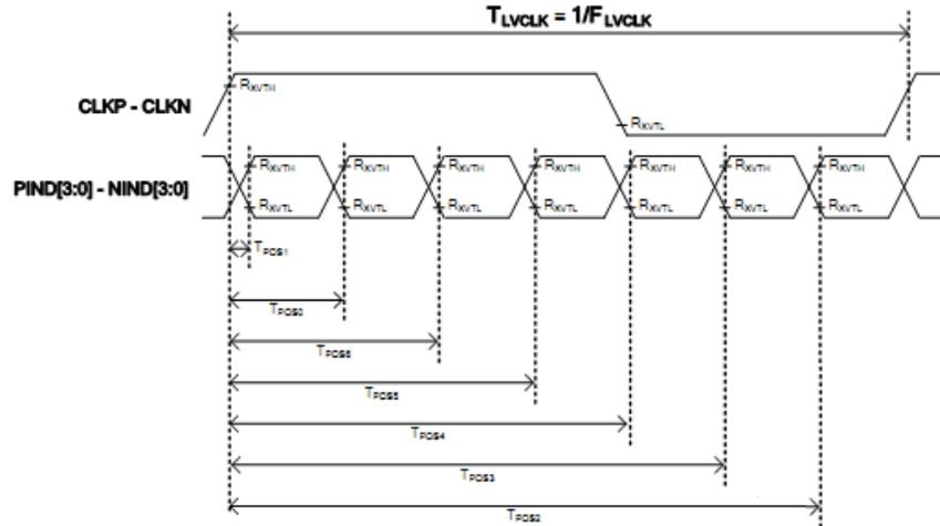
Figure 5.2.3 LVDS input timing
