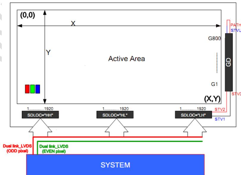
Note: In Dual-Link LVDS mode: The first pixel on panel (top-left) is odd.
