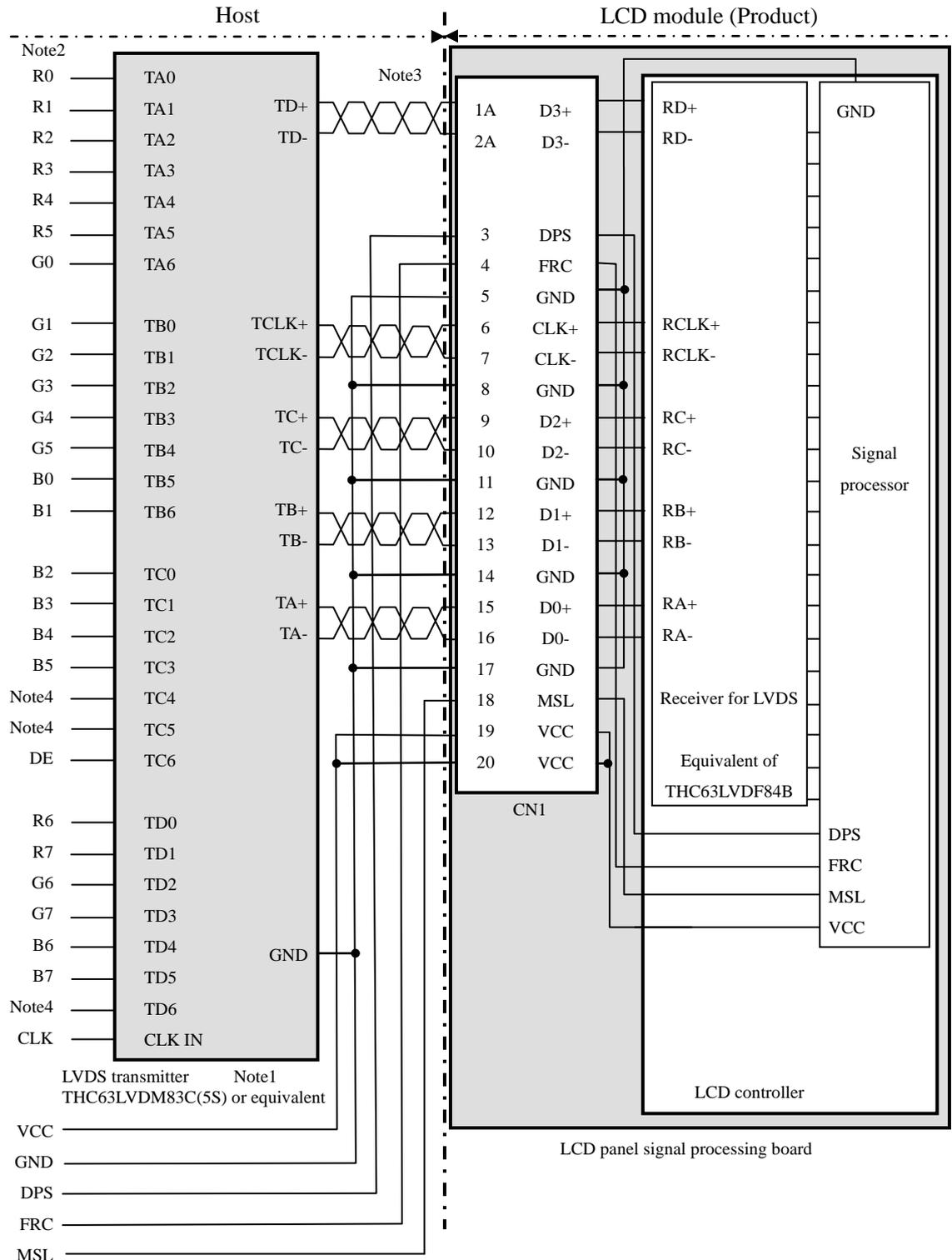
Note1: Recommended transmitter: THC63LVDM83C(5S) (THine Electronics Inc.) or equivalent
