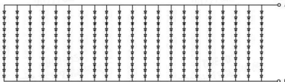
Figure 3-1 Front Light Circuit
