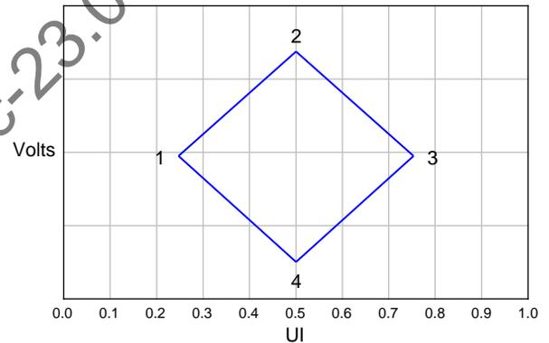
[ EYE Mask at Sink Connector Pins ]
