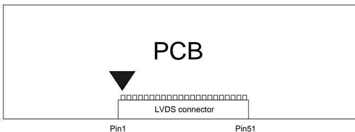
**Note2.** Please leave this pin unoccupied. It cannot be connected with any signal (Low/GND/High).
