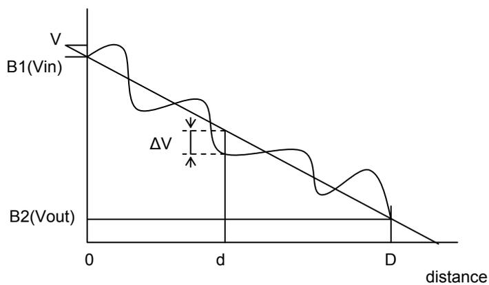
$$LE(\%) = \Delta V / (V_{in} - V_{out}) \times 100$$
