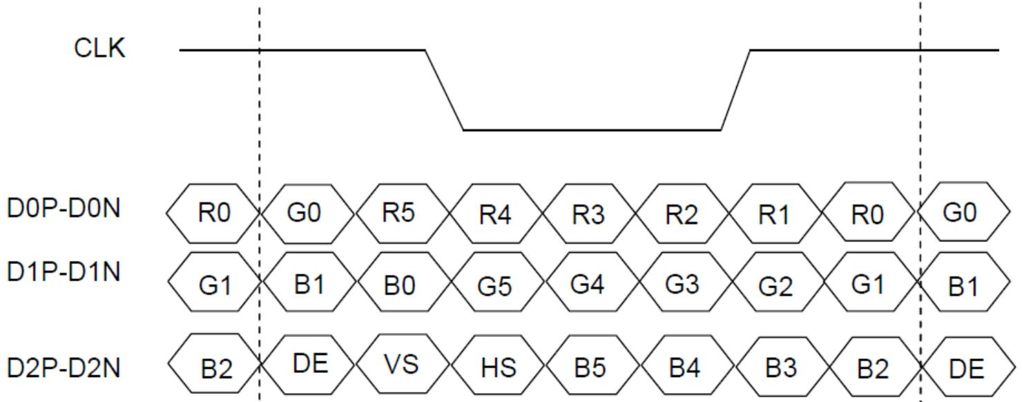
Figure 6.4.1 LVDS data input format (VESA standard)
