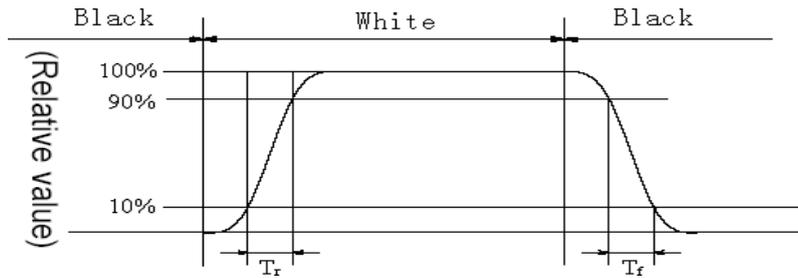
**Fig3. Response Time Testing(SFT)**
