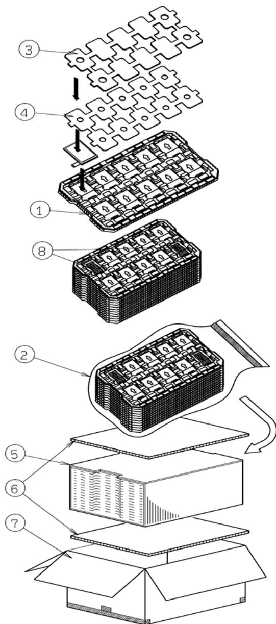
Step 1. Each product is to be placed in one of the cut-outs of the tray with the display surface facing upward. (10 products per tray)
