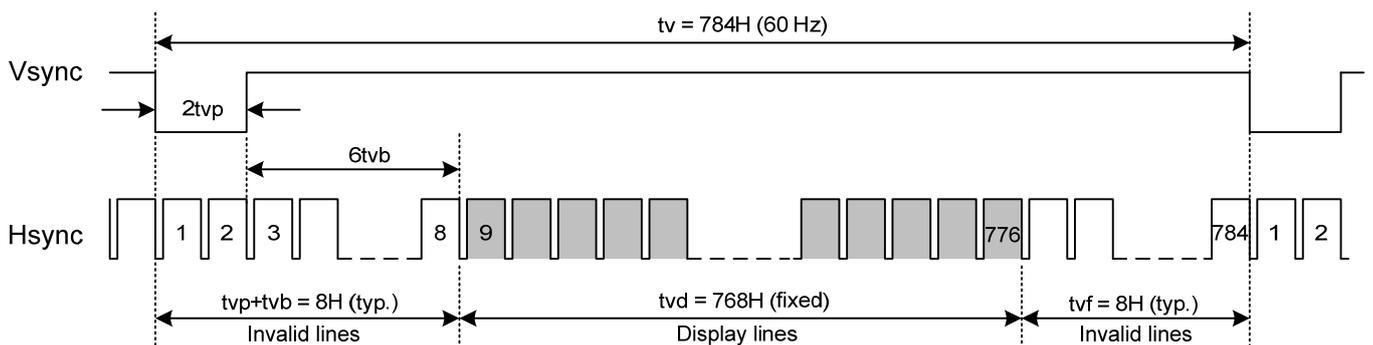
Fig. 9.2 Vertical Timing of Synchronous Mode
