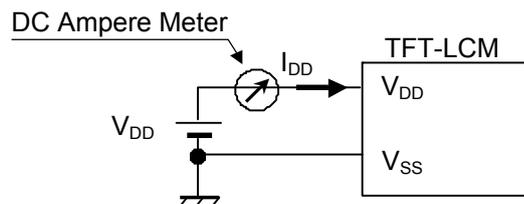
Note 3: 1.5A fuse is applied in the module for  $I_{DD}$ . For display activation and protection purpose, power supply is recommended larger than 3.75A to start the display and break fuse once any short circuit occurred.
