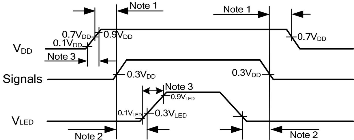
Note 1: In order to avoid any damages,  $V_{DD}$  has to be applied before all other signals. The opposite is true for power off where  $V_{DD}$  has to be remained on until all other signals have been switch off. The recommended time period is 1 second.
