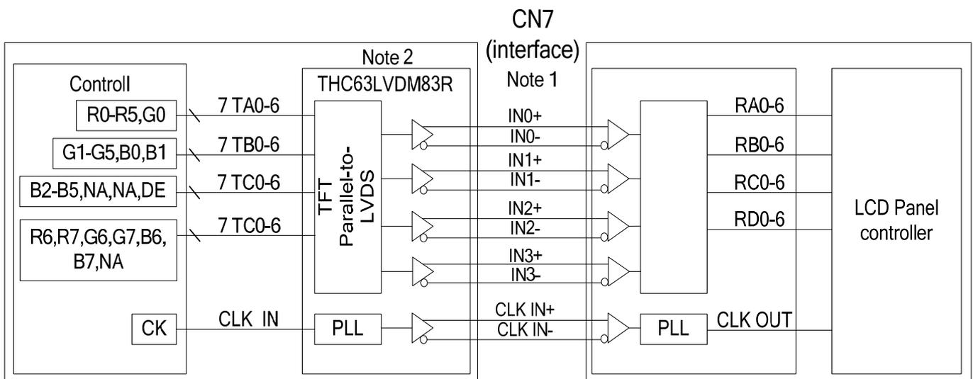
Note 1: LVDS cable impedance should be 100 ohms per signal line when each 2-lines (+, -) is used in differential mode.
