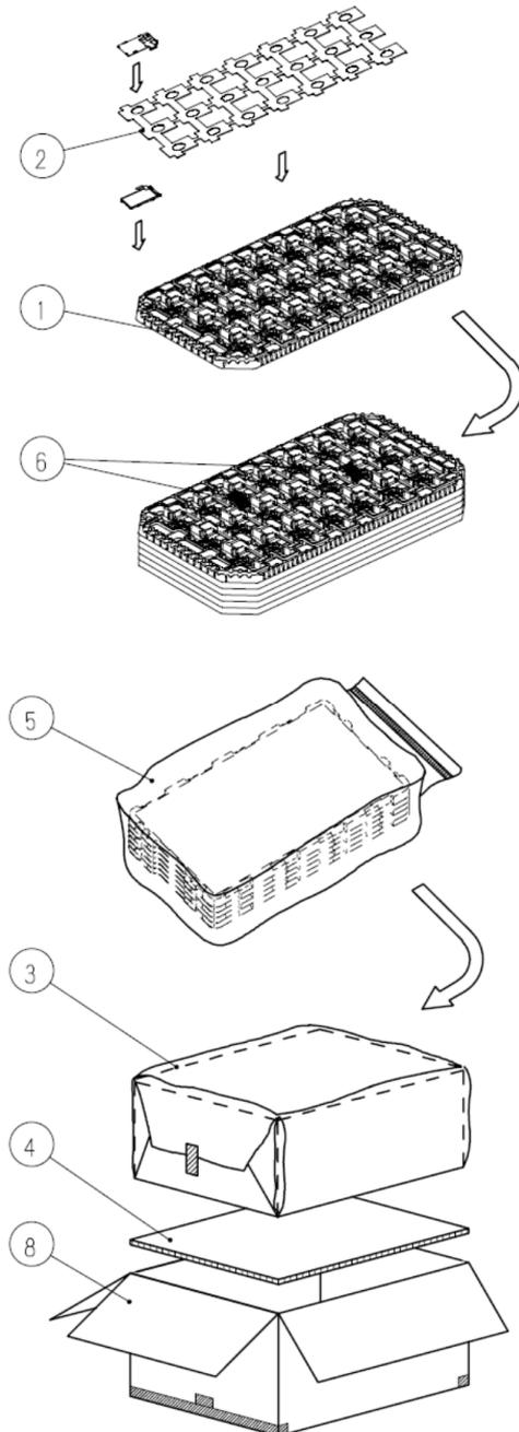
Step1. Each product is to be placed in one of the cut-outs of the tray with it's the LCD display side facing upward,and foam-sheet is put on products.(21 pieces/1 step)
