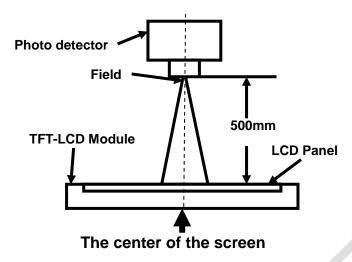
Note 2: Definition of viewing angle range and measurement system. viewing angle is measured at the center point of the LCD.
