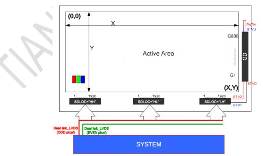
Note: In Dual-Link LVDS mode: The first pixel on panel (top-left) is odd.
