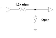
Figure 5.DBC input circuit is as below
