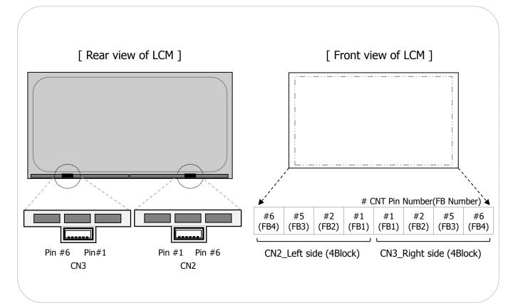
[FIG. 5] Backlight connector view
