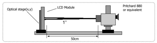
[FIG. 7] Optical characteristic measurement equipment and method
