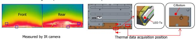
**2)** Measurement of temperature by time. When the temperature is over 63.9 °C on C/Bottom, defects are founded due to thermal effect.
