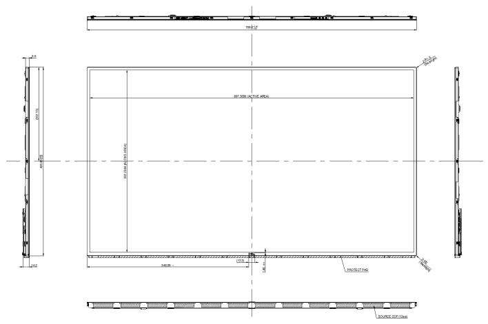
Notes 1. I/F Connector specification: LSMtron, GT05Q-30S-H10-MN or Equivalent 2. LED connector specification: SM06B-SHJH (HF) (Manufactured by JST) or Equivalent 3. Torque of user hole: 3.0~4.0kgf.cm 4. Tilt and partial disposition tolerance of display area as following (1) Y-direction a. Upper side:  $-0.45 \le A \le 0.45$ ,  $-0.45 \le B \le 0.45$  b. Lower side:  $-0.45 \le C \le 0.6$ ,  $-0.45 \le D \le 0.6$  (2) X-direction:  $-0.45 \le E \le 0.45$ ,  $-0.45 \le F \le 0.45$
