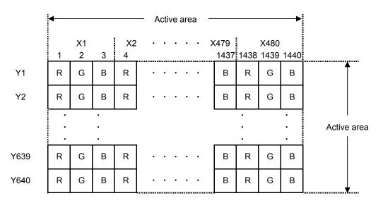
Dot arrangement (FPC cable placed left side)
