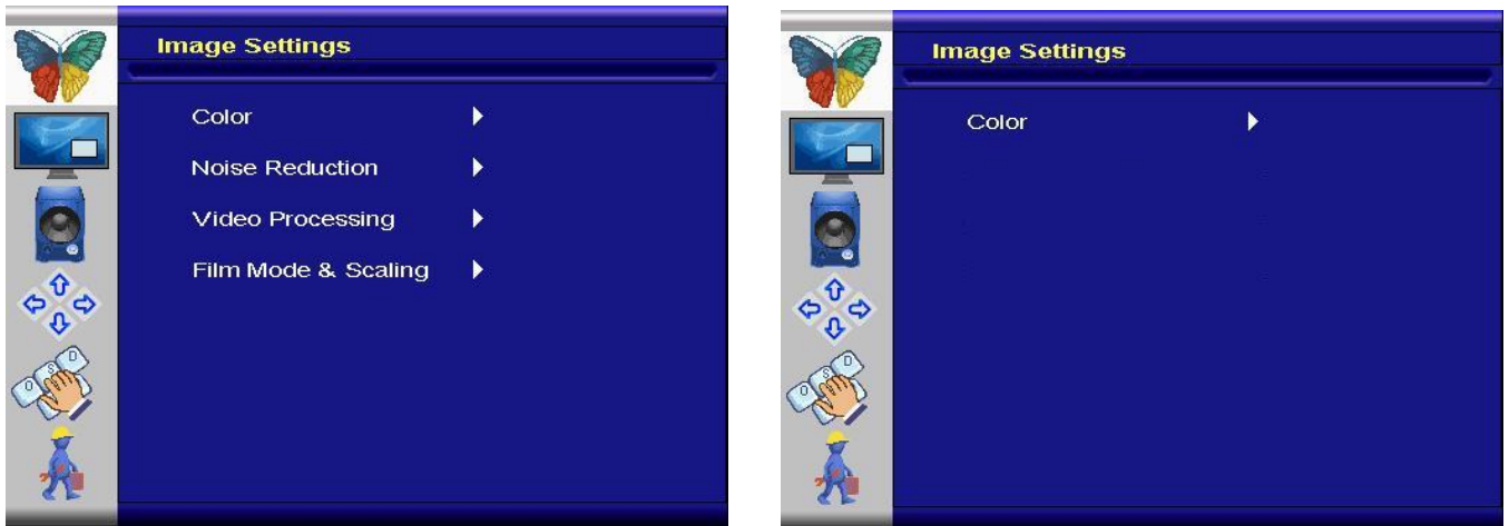
Figure 7.1.c "Advanced" menu for S-Video, CVBS, YPbPr and video mode of DVI/HDMI. Figure 7.1.d "Advanced" menu for VGA and graphics mode of DVI/HDMI.
