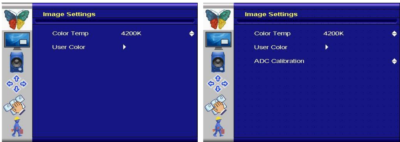
Figure 7.1.e "Color" menu for DVI/HDMI and SDI Figure 7.1.f "Color" menu for S-Video, CVBS, YPbPr, RGB+CS and VGA
